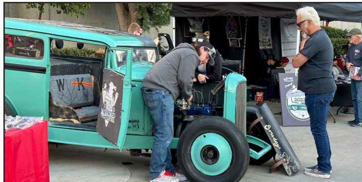
Student Ryan Peters was showing off the custom 1930 model Eh sedan that was built in 6 weeks with a limited budget. Students put in a 1932 chassis, 1932 grill, built new hood and hood sides, built and chopped roof to look like a 1932, changed front axle, hand built intake and exhaust manifold, custom built hubcaps, painted the car, hand painted lettering and numbers that the club displayed at the Grand National Roadster show Feb. 3-5.
