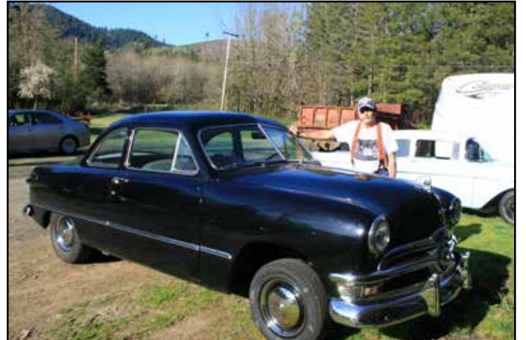
Black Beauty: This black 1950 Shoebox Ford has been owned by Tom Aaron since 1983. Powered by a 239 cubic inch flathead engine, boosted with a Maculloch blower, it is cooled with an aluminum radiator and electric fan. Running a three-speed overdrive transmission and a 1957 nine-inch wagon rear end. Inside, you will find a custom digital dash and instruments to keep track of what is happening. Built by Clarence Everett and painted by David Bazy. (Thank you, Gary Meyer, for the information and photo.)
