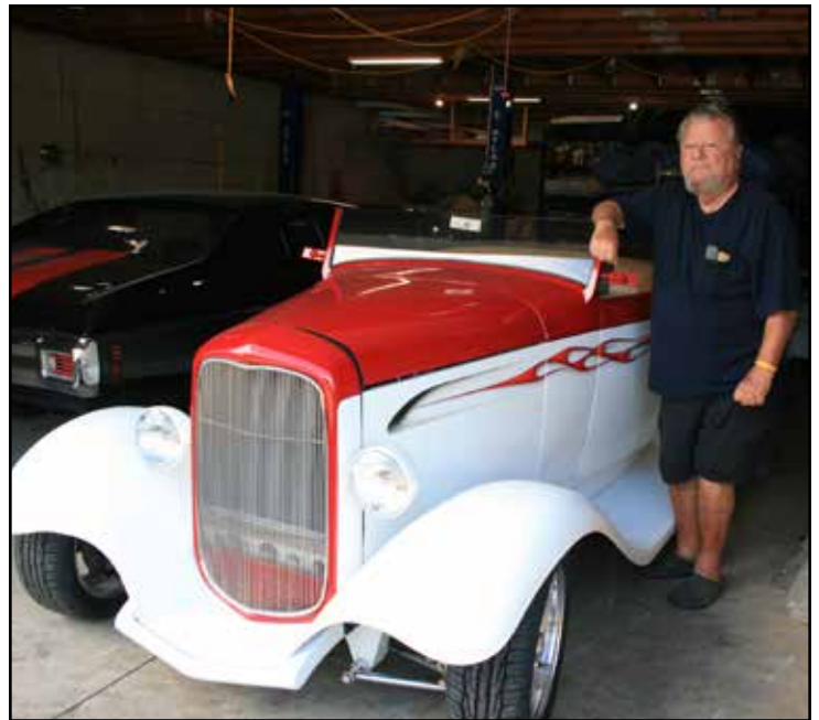
Jon Pierson has owned this show-winning, 1932 Ford Roadster since 1987. The engine is a bored 454 Chevy, built by Trayco of L.A., Calif., makes 518 horse-power. The transmission is a B and M, 400 shifter. A Lincoln Versailles rearend transfers the power to the aftermarket wheels and tires. The front end is from Kuggle with independent suspension. (Photo and information courtesy of Gary Meyer.)
