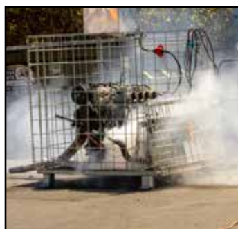
The engine blowout didn't last long, as it threw chunks of the flywheel 30 seconds into full-out revving of the engine.
