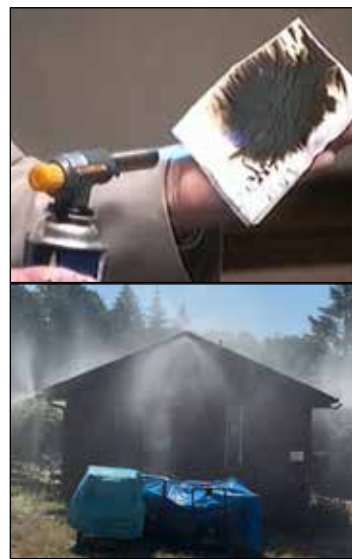
Top: A white napkin treated with one of Hoffmann's fire protection products chars when exposed to flame but does not catch fire. Bottom: Hoffmann's exterior sprinkler system sprays water around a structure during a demonstration.
